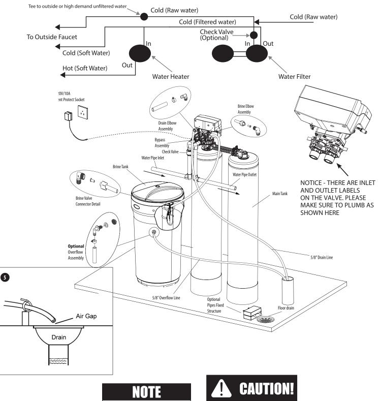
Waste connections or drain Never insert drain line outlet shall be designed and directly into a drain, sewer constructed to provide for line, or trap. Always allow an connection to the sanitary air gap between the drain waste system through an line and the wastewater to air-gap of 2 pipe diameters prevent the possibility of or 1 inch (22 mm) whichever sewage being back-siphoned is larger. into the conditioner.
