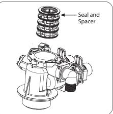
5. Replace piston assembly followed by timer assembly.6. Replace the piston assembly and reverse following steps in this section
