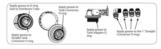
Ensure all Oring on both tank connectors are properly dissembled and apply a good amount of grease.
