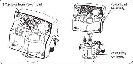
5. Remove the two screws from the powerhead as shown6. Life the powerhead from the valve body assembly7. Replace the powerhead by reverse following the steps in this section
