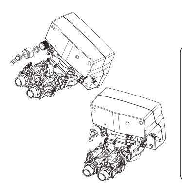
Install the connectors with fitting as shown. Also install the valve on the parallel adaptor.
