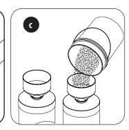
c) Fill support bed first. The media will not always spill down inside the tank and may need to be swept inside.
