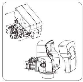
1. Remove the screws from the back of the valve and pull the front cover
