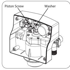
4. Remove the piston screw and washer from the piston rod.
