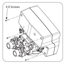
2. Remove four screws from the back of the valve cover
