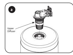
a) Remove the adaptor from the mineral tank. Grease the bottom oring of the adaptor with silicone grease provided
