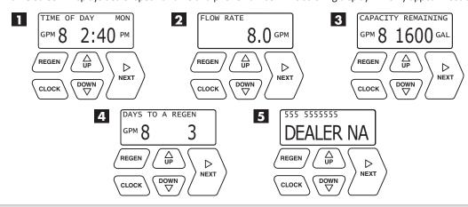
If the system has called for a regeneration that will occur at the preset time of regeneration, the words "REGEN TODAY" will appear on the display. If a water meter is installed, "GPM" flashes on the display when water is being treated, indicating gallons per minute flowing through the system.
